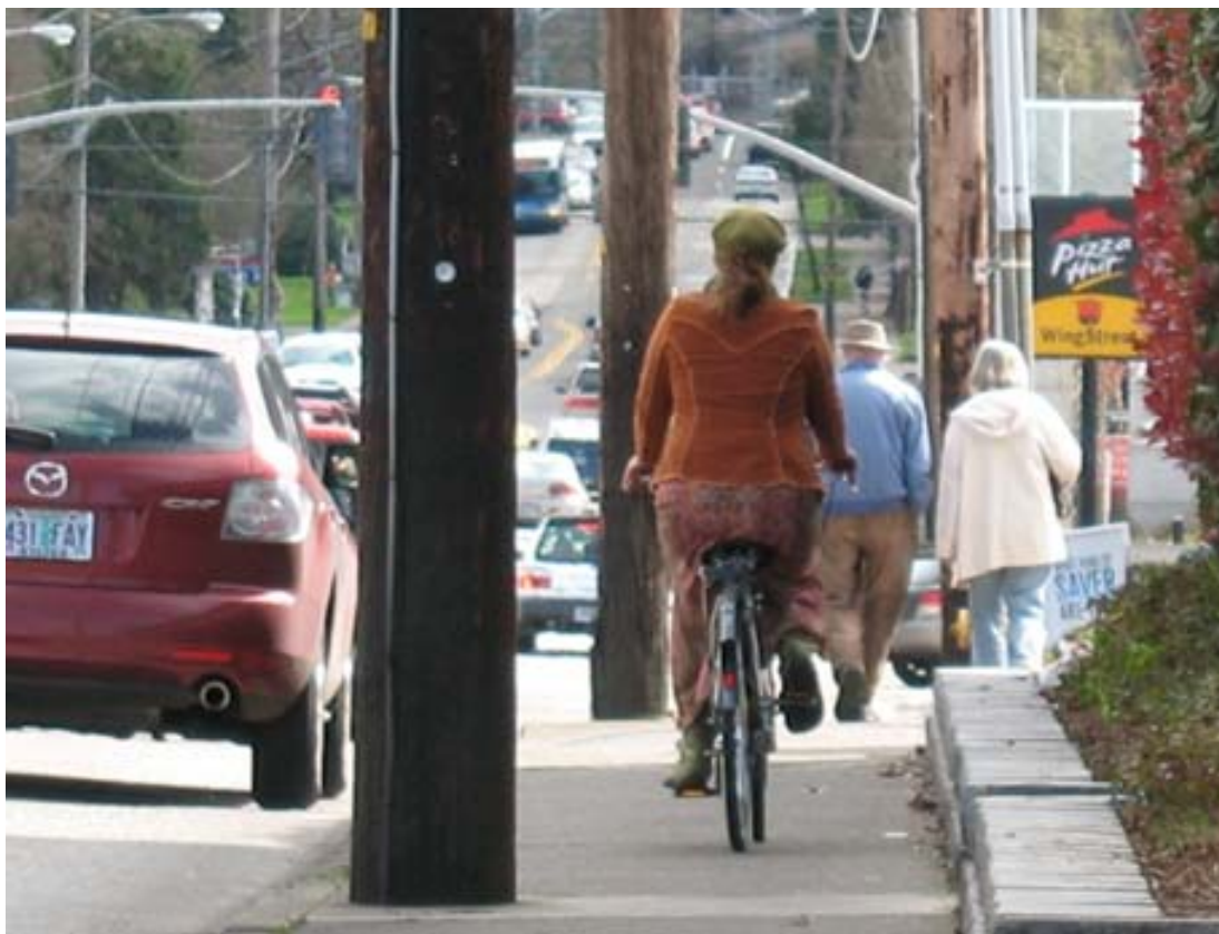
Sidewalks on South Willamette Street are generally narrow with numerous obstructions, no separation from travel lanes, and a mixture of pedestrian and bicycle traffic.
