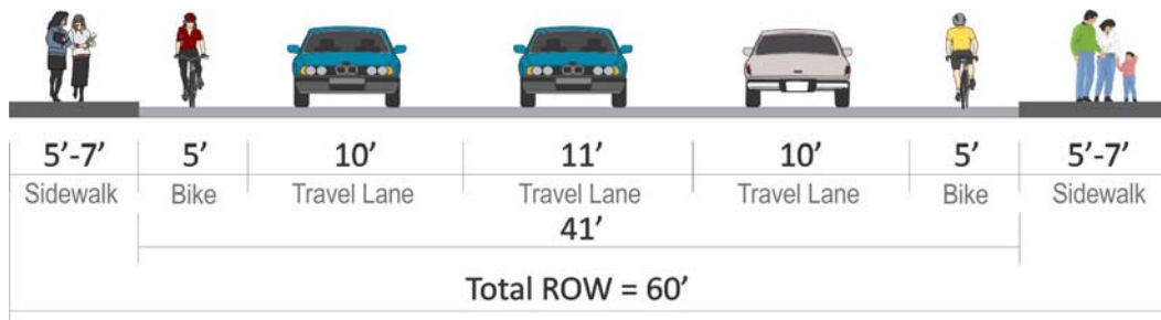
Figure 2c: 3-Lane Cross Section (South of 29th Avenue)
