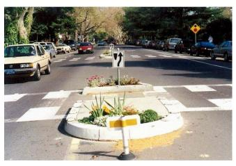
Median pedestrian crossing refuges provide a waiting area for a two-stage pedestrian crossing.
