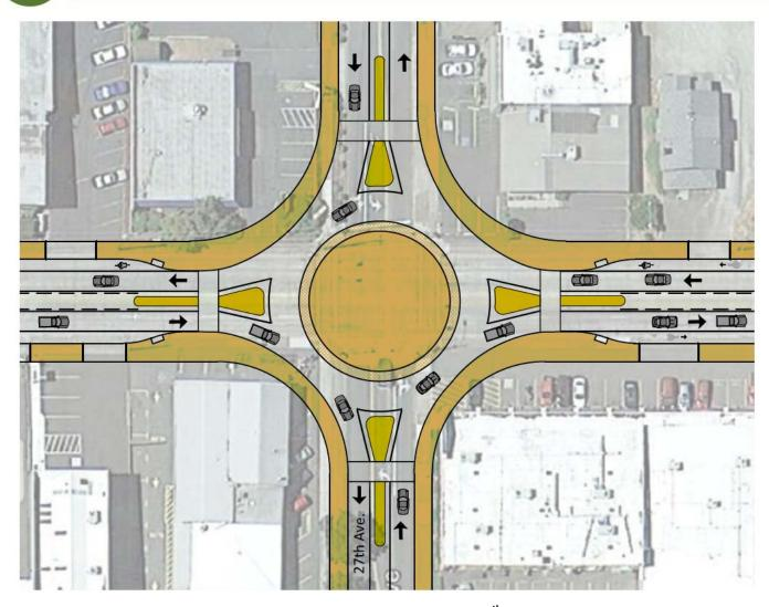
Figure 21: Potential Single-lane Roundabout Configuration at 27<sup>th</sup> Avenue and Willamette Street
