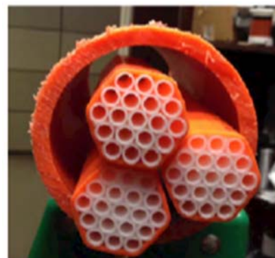
Microduct-the fiber lies in the small white, 'honeycomb' tubes.
