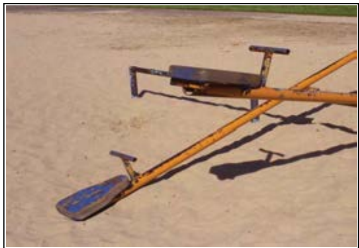
Sand in playground areas is inaccessible to wheelchairs and can create safety issues.
