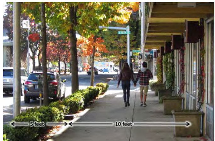
Example of wide sidewalk with planting buffer, street trees, and on-street parking .
